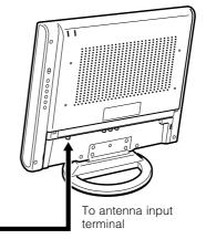
75-ohm coaxial cable (round cable)
